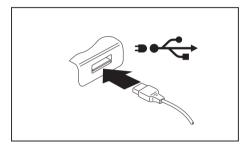
You can use this USB port to charge or supply power to a USB device (e.g. to charge a PDA or a mobile phone or to connect a USB lamp), even if the notebook is switched off.
